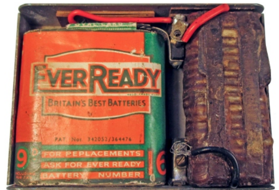
Battery box with an original 4.5V LT and 30V HT battery.
