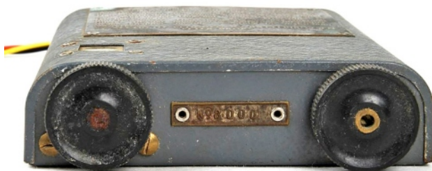
Front panel (above) and rear panel view (below). Note the typical Brush hearing-aid earphones socket at the left hand side of the rear panel.
