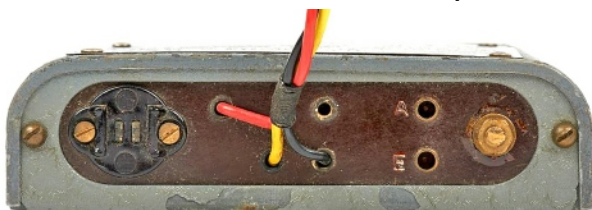
Front panel (above) and rear panel view (below). Note the typical Brush hearing-aid earphones socket at the left hand side of the rear panel.
