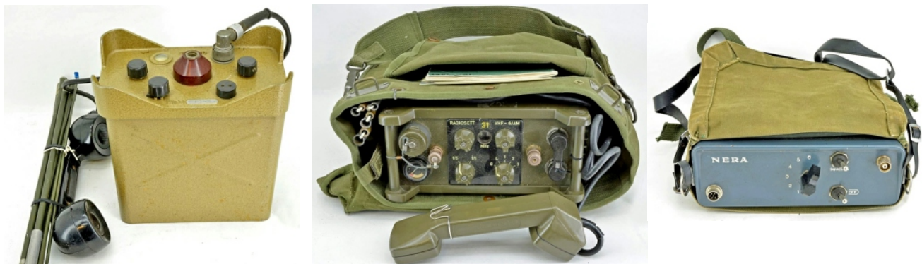
Later produced Simrad man-pack transceivers for the Norwegian Army were the W.T.3 (left) and the VHF-6AM (centre), both amplitude modulated, operating on 30MHz. The man-pack radio at the right was a W.T.2 A made by NERA, which was a later transistorised replacement of the Simrad W.T.2.
