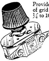
Provides a noiseless range of grid leak resistance from  $\frac{1}{4}$  to 10 megohms. Assures most effective grid leak resistance value for *all* tubes. Small grid condenser (0.00025) is separate. Metal parts nickel plated. One hole mounting.
