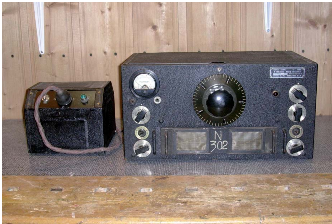
R-106/HRO mottaker m/power supply. Laget for British Government 1944.
